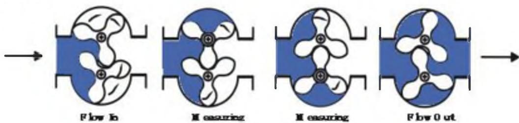
LSZQ Series Gas Double Rotator Flowmeter classified into two groups:
